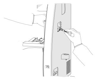
12. Remove the coolant tubing from the notched arm.
