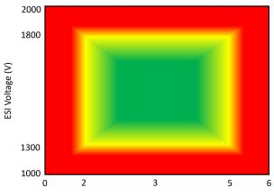
Figure 6-11 Sprayer Tip Distance and ESI Voltage Correlation
