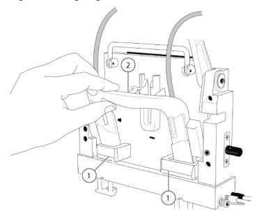
Figure 3-5 Aligning Blocks
