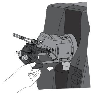
CAUTION: Potential System Damage. Move the stage before the adapter is installed on the mass spectrometer. During the installation of the sprayer assembly, the glass tip of the sprayer is exposed. If the ion source stage is too close to the inlet on the mass spectrometer, then damage to the sprayer tip can occur. 3. Install the adapter in the ion source and push the adapter as far forward as possible, so that the hook at the end of the adapter goes under the end of the rail.
