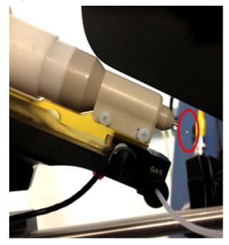
**Note:** If the separation capillary is empty, then the first droplet of solution might not show at the sprayer tip for as long as 7 minutes.
