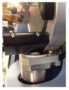
Figure 3-33 Cover on the Source Drain Assembly
