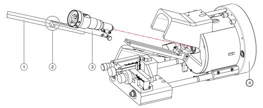
Figure 3-26 Orientation of the Adapter Before Installation
