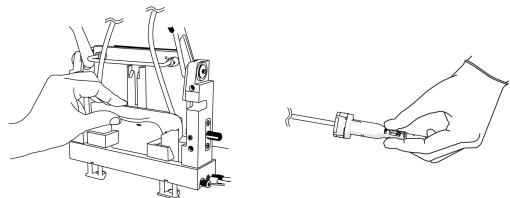
**Note:** As the cartridge is moved up, the sheaths on the inlet and outlet sides go down over the capillary ends.
