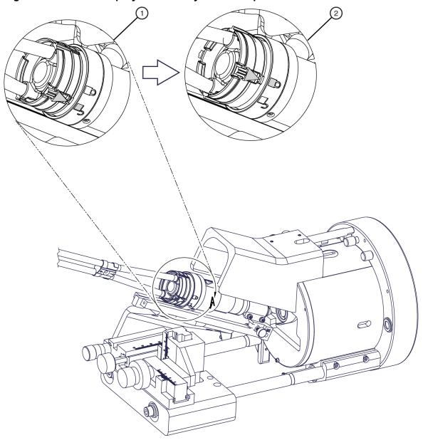
Figure 3-30 Lock the Sprayer Assembly in the Adapter
