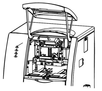
2. Loosen the thumbscrews on the insertion bar, and then lift the insertion bar.
