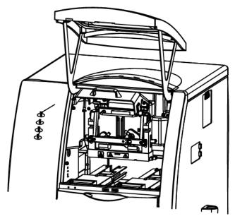
The coolant pump for the CESI 8000 Plus system turns on and releases the coolant from the cartridge coolant lines. Approximately 30 seconds are required. Wait for the pump to turn off.
