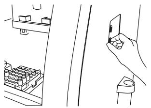
4. Put the sprayer housing through the side panel, and then put the sprayer in the holster.
