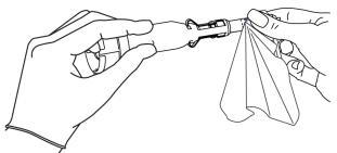
CAUTION: Potential System Damage. To prevent the sprayer tip from breaking, do not move the retractable protective guard during drying.
