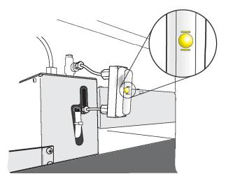
6. Remove the coolant fill tool, and then close the sample cover.
