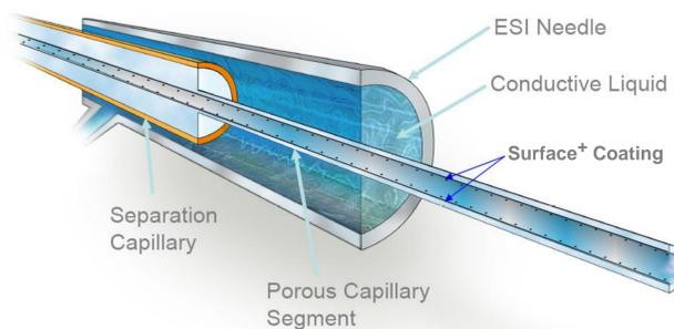
Figure 3: OptiMS CESI Interface Schematic
