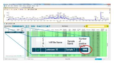
Figure 1. Non-targeted (unknown) screening and identification; Nontarget XIC generation using a non-targeted peak finding algorithm will find thousands of molecular features in a sample. Only a handful will be significant components.
