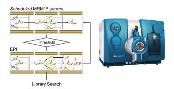
Figure 1. The QTRAP® 4500 system was employed with EPI scan type triggered by signal from target pesticides monitored in MRM mode. The resulting MS/MS spectrum were matched to library spectra for confirmation.
