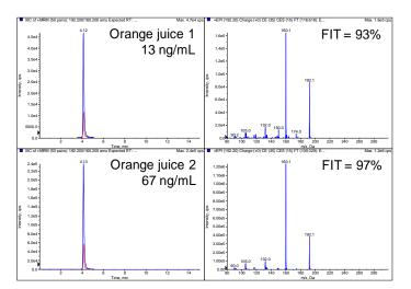
**Figure 6.** Identification of Carbendazim in two orange juice samples using MS/MS library searching: The samples were injected directly after 5x dilution, and FIT values above 90% clearly confirm the identity of Carbendazim.
