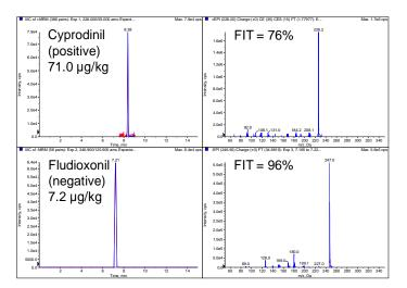
**Figure 7.** Identification of Cyprodinil and Fludioxonil in a raspberry sample using MS/MS library searching: The samples were injected after QuEChERS extraction and 5x dilution, and MS/MS spectra were acquired in positive polarity and negative polarity.
