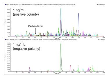
**Figure 1.** Comprehensive pesticide screening using the *Scheduled* MRM<sup>™</sup> algorithm and fast polarity switching, ~500 MRM transition were detected with a total target cycle time of 0.7 sec
