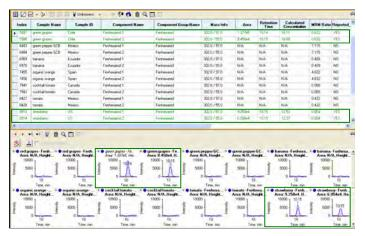
**Figure 4.** Automatic reporting of pesticides using the 'Multicomponent' query in MultiQuant<sup>™</sup> software: Fenhexamid was positively identified using MRM ratio calculation in two samples and quantified in green grapes at 18.1 µg/kg and in strawberry at 12.5 µg/kg, respectively.
