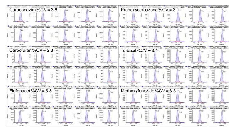
**Figure 2.** Repeat injections of pesticides at a concentration of 1 ng/mL detected in positive (left) and negative (right) polarity in a single run using *Scheduled* MRM<sup>TM</sup> and fast polarity switching (Carbendazim and Propoxycarbazone at 4.1 min, Carbofuran and Terbacil at 6.1 min, and Flufenacet and Methoxyfenozide at 10.3 min)
