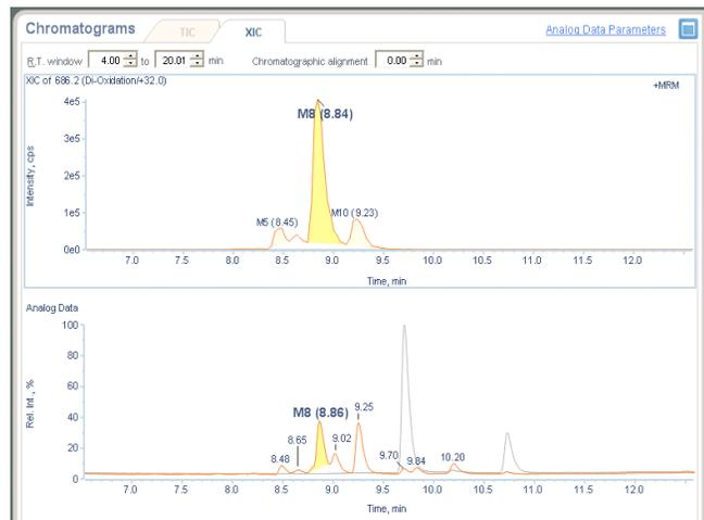
**Figure 5. The selected ion chromatogram for the di-oxidation metabolites of bromocriptine (top) and the UV chromatogram (bottom).**
