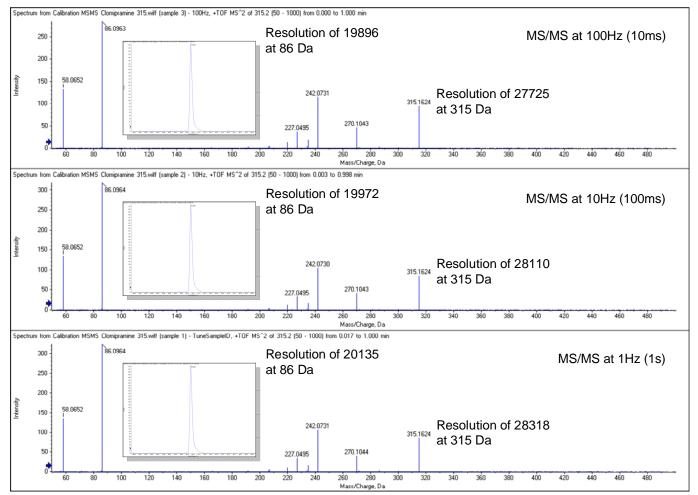
Figure 1. Highest resolution at every scan speed over the entire mass range with stable mass accuracy of ~1 ppm
